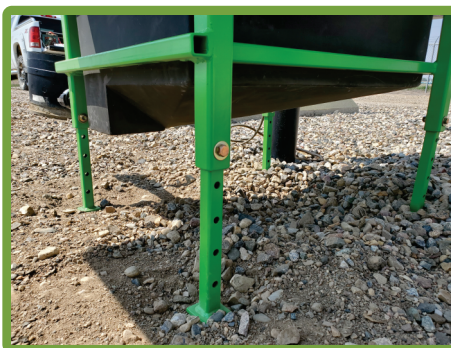
Adjustable legs, helping to position the container close to the pipeline
